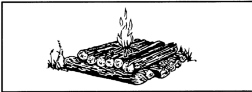
Figure 7-3. Base for fire in snow-covered area.
