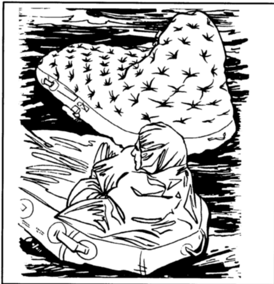
Figure 16-11. One-man raft with spray shield inflated.
