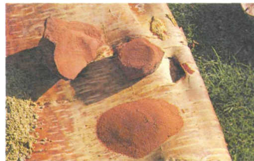
Burned and ground sandstone for use as temper.
