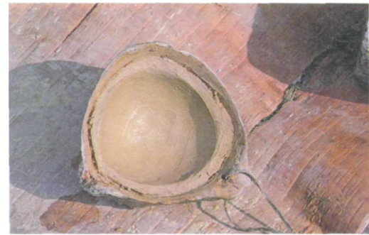
Moulding a clay bowl in a wooden mould.
