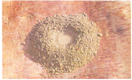
Dried and crushed clay, with temper added, being mixed with water.
